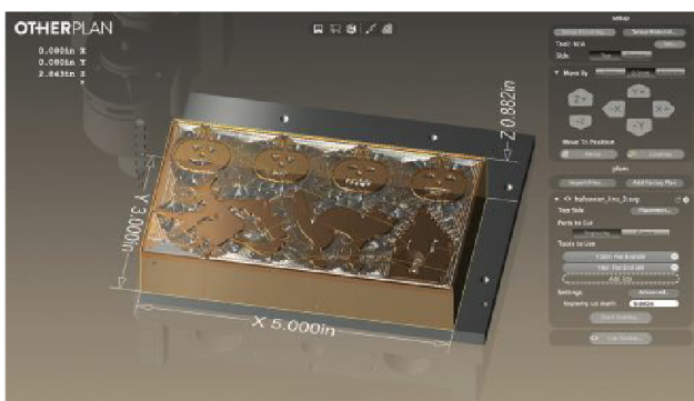
Otherplan, the CAM software from Other Machine Co., shows a toolpath preview for an intricate Halloween stamp. Image courtesy of Other Machine Co.
