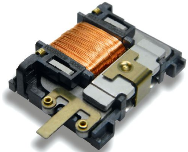
An electromechanical harvester for kinetic power. Image courtesy of EnOcean.
