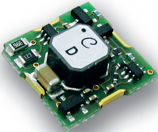
A DC/DC converter for thermal power. Image courtesy of EnOcean.
